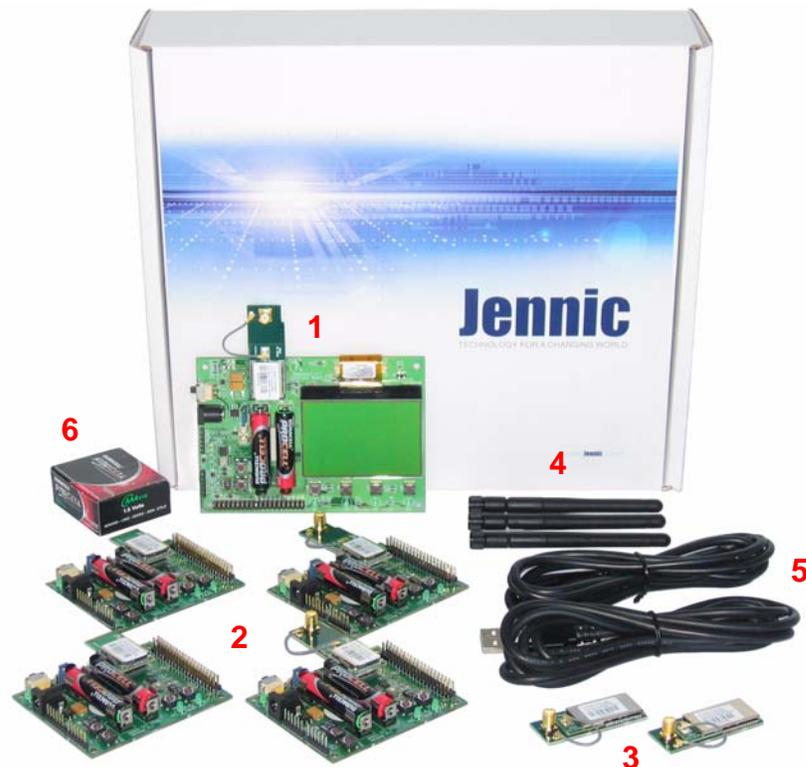
**Figure 1: JN5148-EK010 Evaluation Kit Components**
