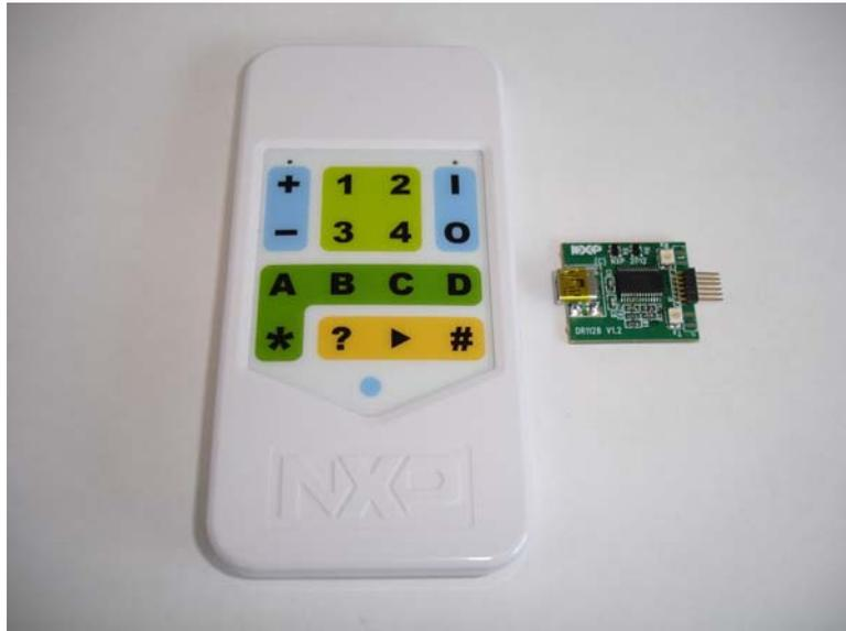
Figure 5: DR1159 Remote Control Unit (and DR1128 Programming Dongle)
