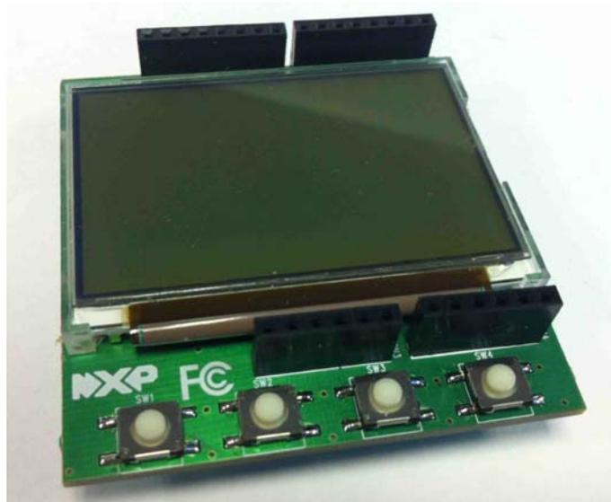
Figure 17: DR1201 LCD Expansion Board
