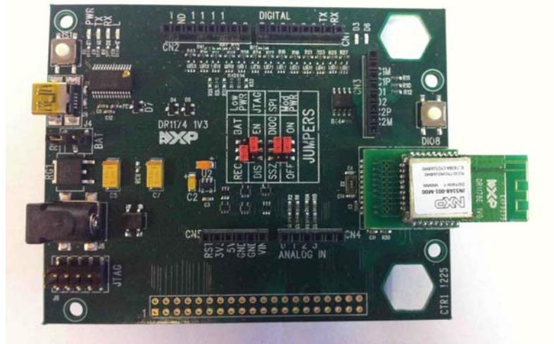
Figure 7: DR1174 Carrier Board (with a JN516x Module)
