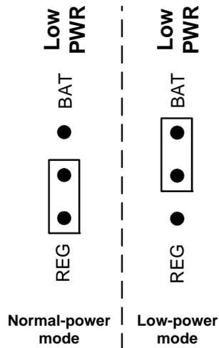
Figure 10: Lower-Power Mode Selection (using Low PWR Jumper)
