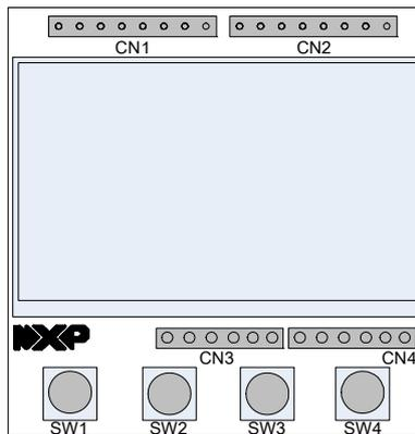
Figure 16: DR1201 LCD Expansion Board Layout
