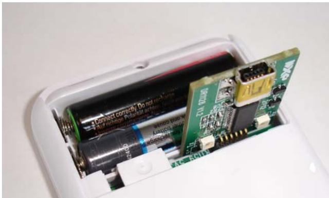
3. Use one of the supplied 'USB A to Mini B' cables to connect the USB Mini B port on the Programming Dongle to a USB port of your PC (you may be prompted to install the device driver for the FTDI chip which is located on the dongle - if this is the case, refer to [Appendix B.4](#)).
