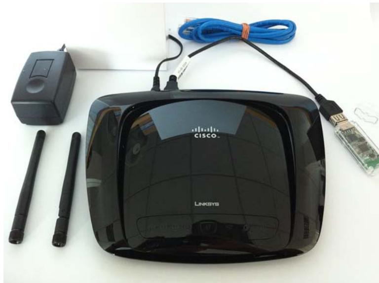
**Figure 22: Linksys Router and Accessories**
