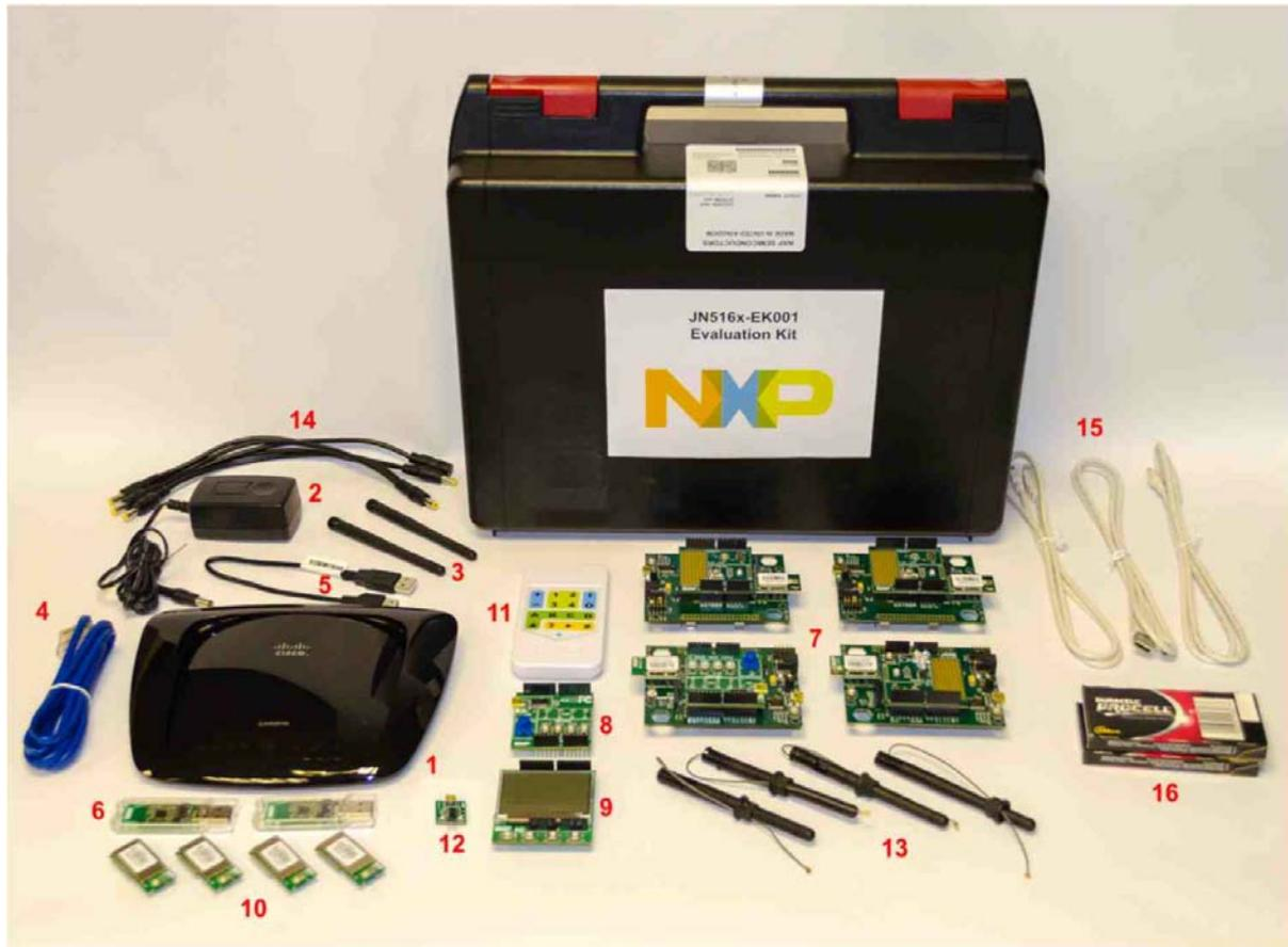
**Figure 4: JN516x-EK001 Evaluation Kit Components**
