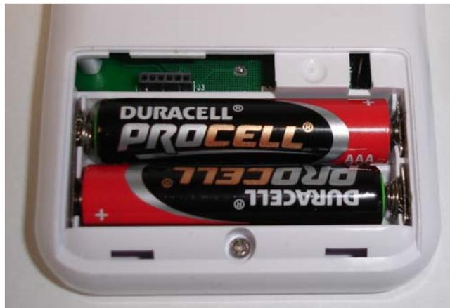
2. Insert the Programming Dongle onto the header in the battery compartment, as illustrated below.
