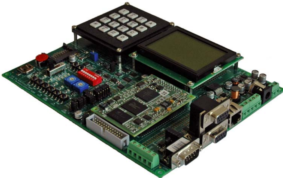
Figure 2: Development Kit PLCcore-5208
